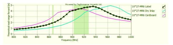
Sensitivity&Read Range Test power: 4W EIRP
